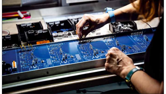
Conventional components – i.e., those with wire connections – are assembled by hand
