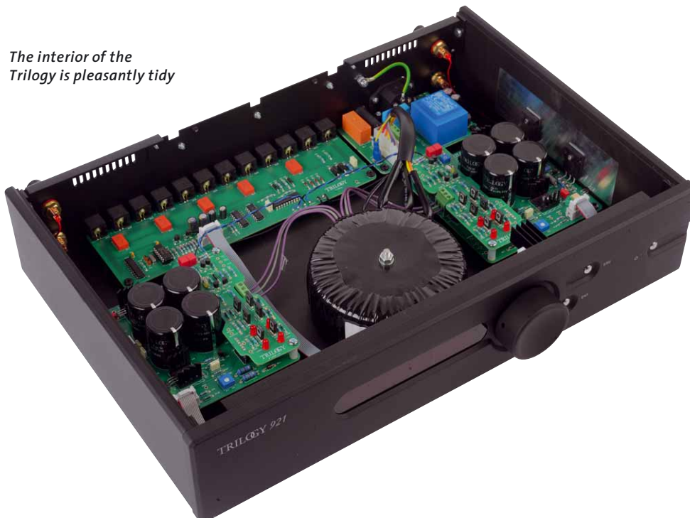
The long chip in the center of the image is the volume control
