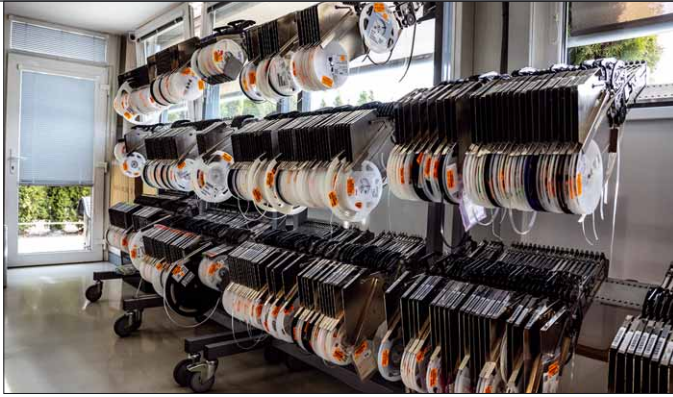
SMD components? Canor has plenty of them, and the circuit boards are naturally also assembled in-house
