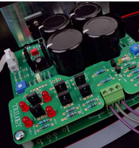
The power amplifier plug-in board contains the complete voltage amplification
