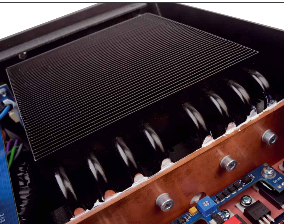
The cooling concept uses heat pipes for heat dissipation
